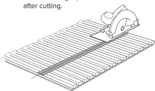
2. Lay the panel flat and mark the cut line.
